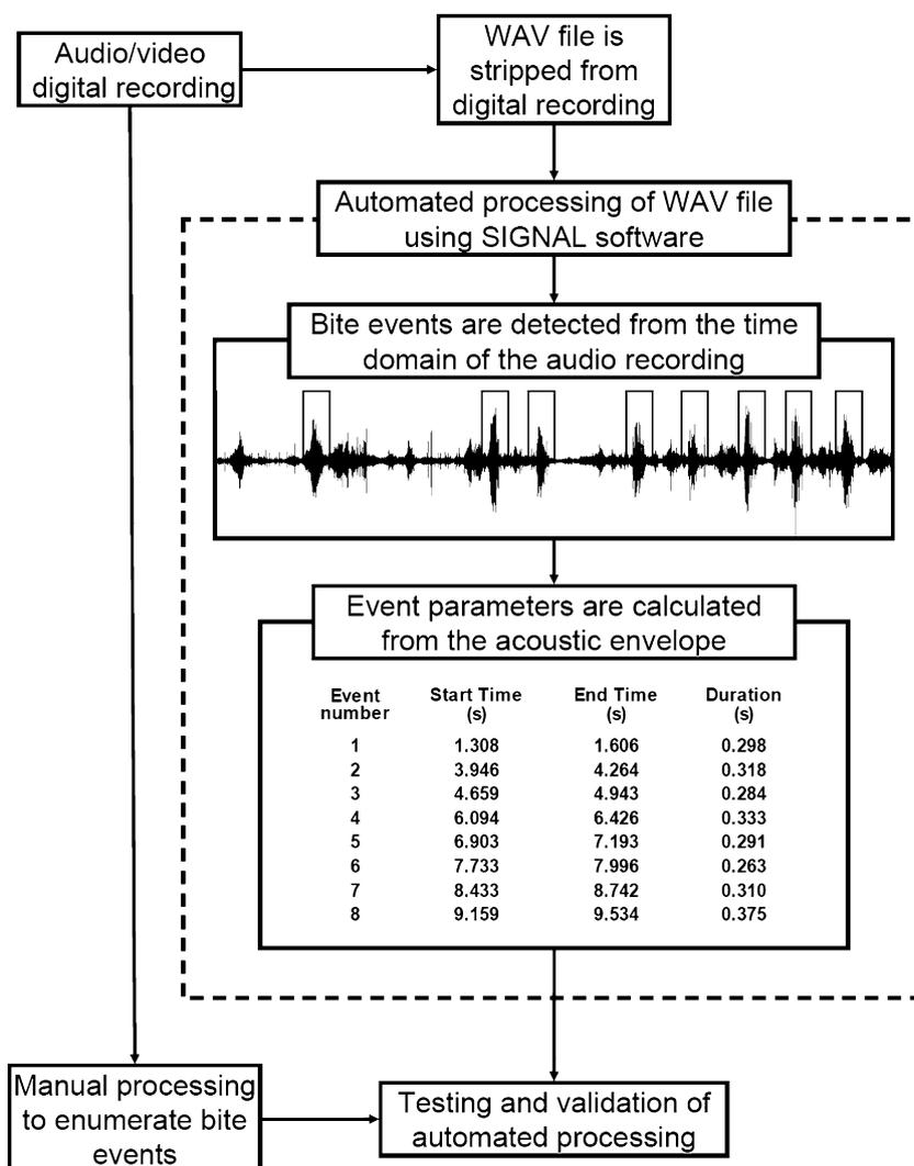
**Fig. 2.** Schematic of testing and validation procedure for automated processing of audio recordings. The waveform represents acoustic pressure over 10 s, recorded from steer 751 while grazing mixed pasture on July 28, 2005. Rectangular boxes on the waveform mark bite events detected by the SIGNAL program. Measured event parameters are shown in the box below the waveform, as an example of program output.
